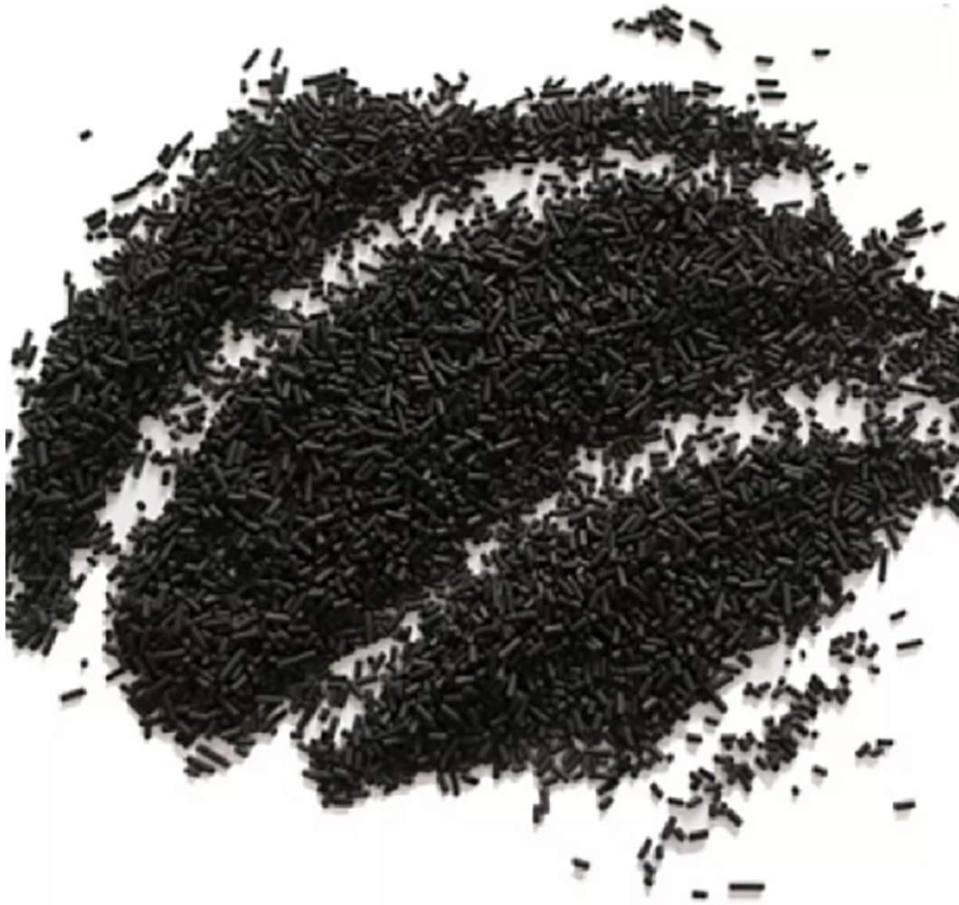
Figure 116: Activated Carbon Pellets from Coal COURTESY OF XINGSHI ACTIVATED CARBON
