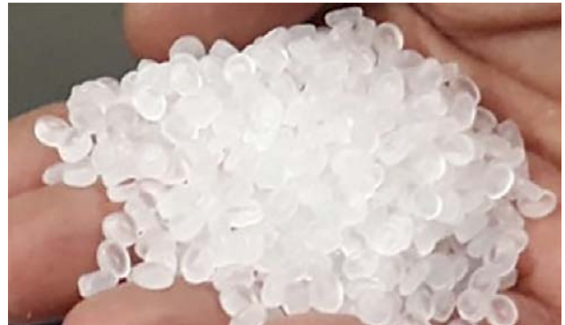
Figure 115: Polypropylene Molecular Structure (Left) and Pellets (Right)
