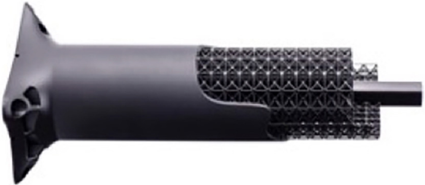
Figure 120: 3D Carbon Fiber Solid Lattice that Could be Made from Coal COURTESY OF RAMACO CARBON
